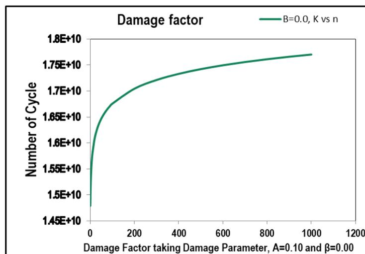
Figure 4. Model prediction of Damage Factor with number of cyclic loading. Adopting the Value of Fatigue Damage Parameter,  $A=0.10$  and  $\beta = 0.00$
