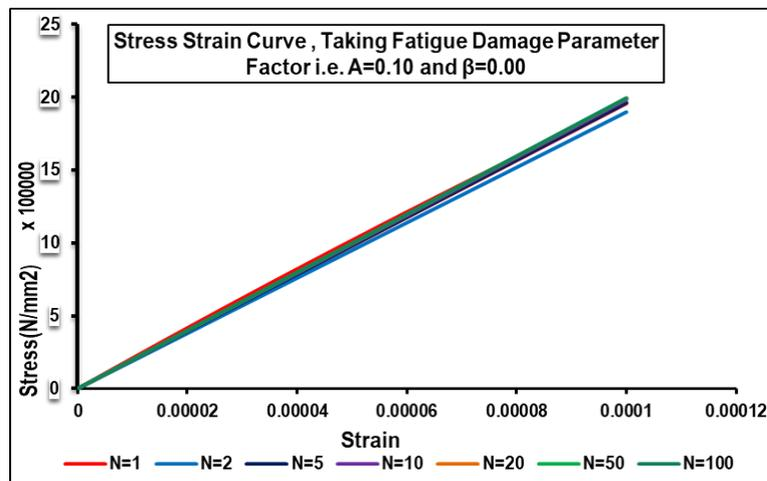
Figure 6. Theoretical cyclic stress-strain behaviour of concrete during elastic damaging process under uniaxial fatigue loading. Adopting the Value of Fatigue Damage Parameter,  $A=0.10$  and  $\beta = 0.00$
