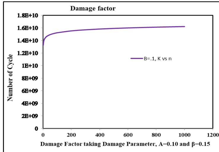
Figure 5. Model prediction of Damage Factor with number of cyclic loading. Adopting the Value of Fatigue Damage Parameter,  $A=0.10$  and  $\beta = 0.15$
