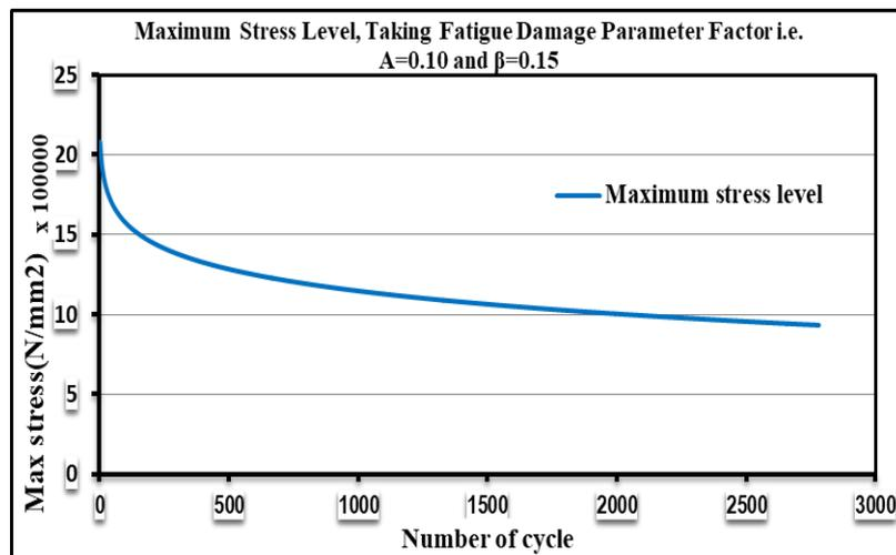
Figure 9. Model prediction of Maximum Stress Level versus Number of Cycle under uniaxial fatigue loading. Adopting the Value of Fatigue Damage Parameter,  $A=0.10$  and  $\beta = 0.15$
