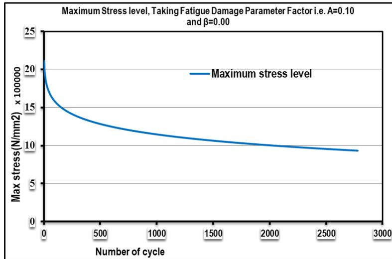
Figure 8. Model prediction of Maximum Stress Level versus Number of Cycle under uniaxial fatigue loading. Adopting the Value of Fatigue Damage Parameter,  $A=0.10$  and  $\beta = 0.00$
