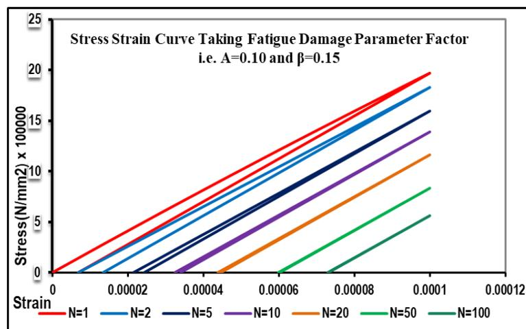
Figure 7. Theoretical cyclic stress-strain behaviour of concrete during elastic damaging process under uniaxial fatigue loading. Adopting the Value of Fatigue Damage Parameter,  $A=0.10$  and  $\beta = 0.15$
