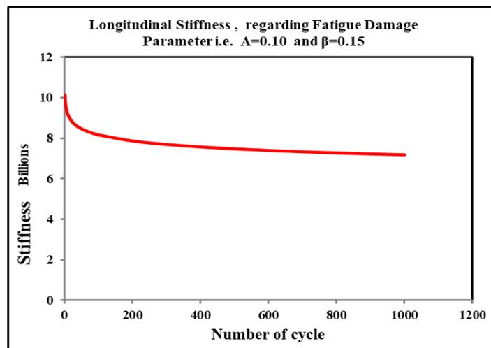
Figure 3. Model prediction of stiffness reduction with number of cyclic loading. Adopting the Value of Fatigue Damage Parameter,  $A=0.10$  and  $\beta = 0.15$
