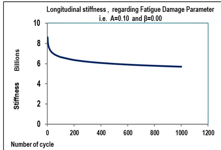
Figure 2. Model prediction of stiffness reduction with number of cyclic loading. Adopting the Value of Fatigue Damage Parameter,  $A=0.10$  and  $\beta = 0.00$
