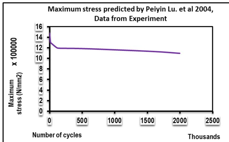
Figure 10. Reduction in maximum stress level during cyclic tension. Prediction of the theory, Figure 8 and 9 by Peiyin Lu. Et. A1 2004
